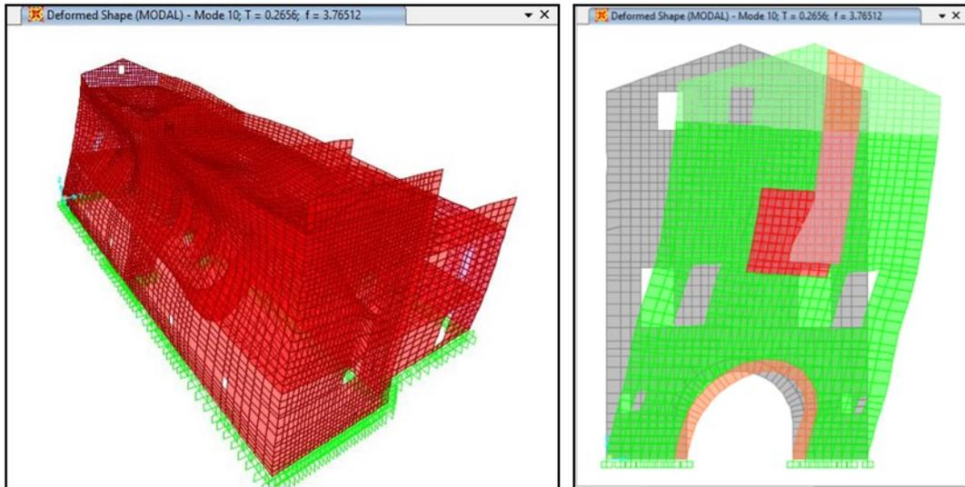
Fig. 2. First modal form for the whole structure and for the intermediate wall with the wall panel (© authors).
