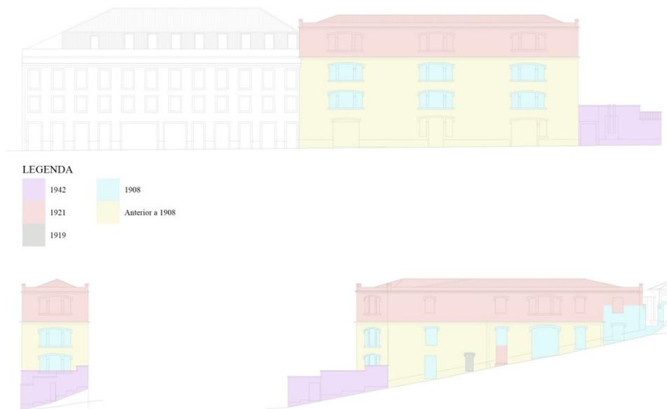
Fig. 2. Stratigraphic reading of one of the sectors of the convent (© Tiago Cruz).
