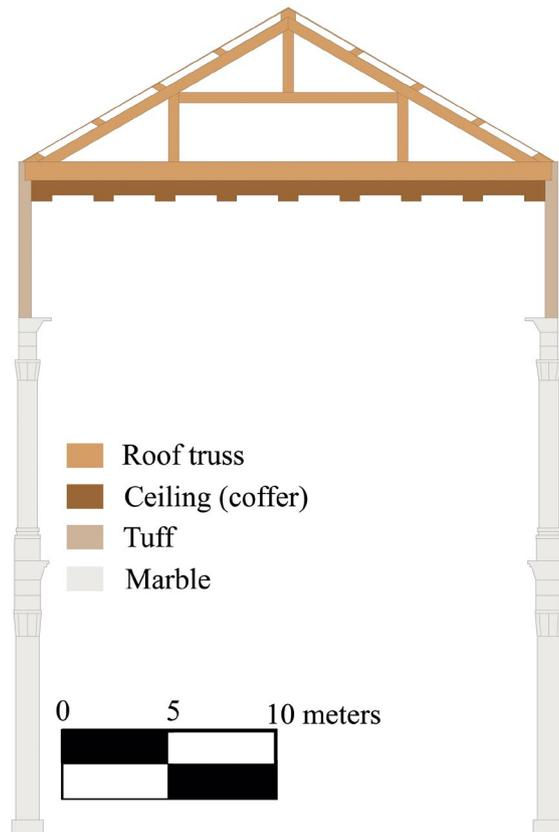
Fig. 1: Reconstructed section of the Basilica Ulpia.
