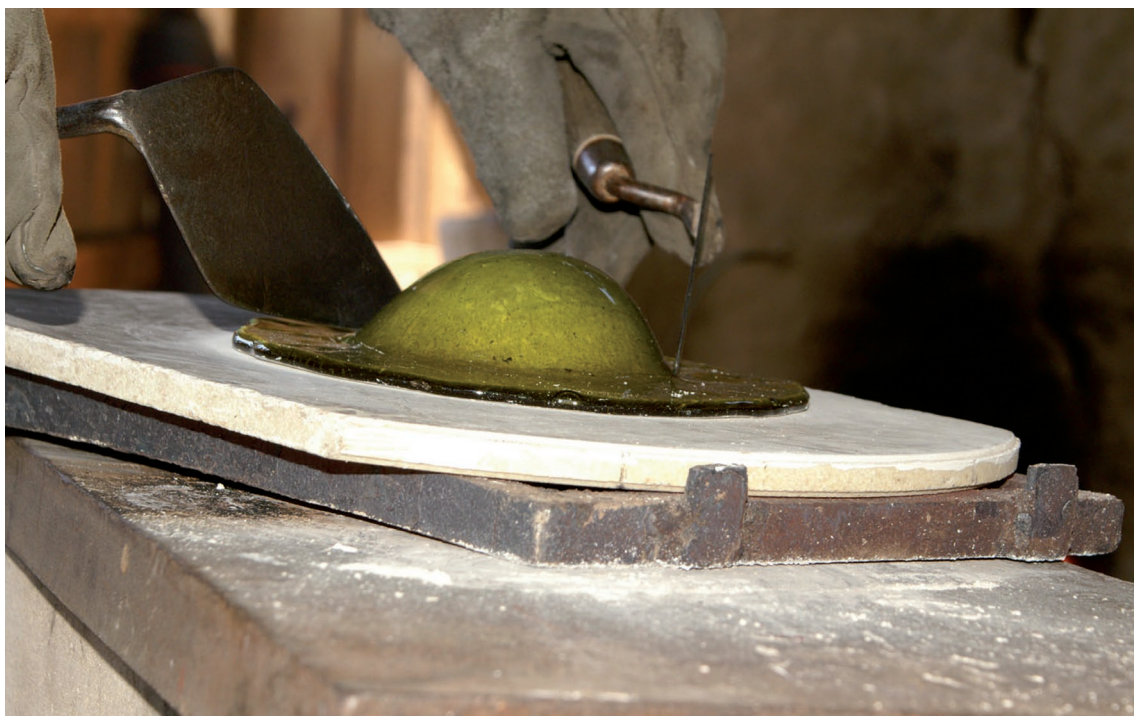
Fig. 8: Last corrections of the domed window glass.
