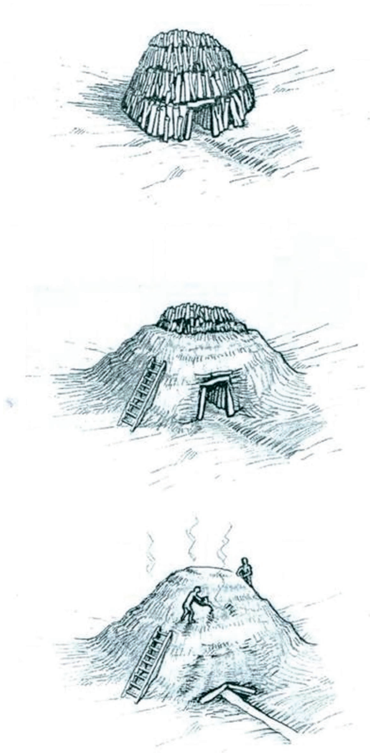
Fig. 3: Reconstruction of the Theophrastean pitch kilns of Macedonians.
