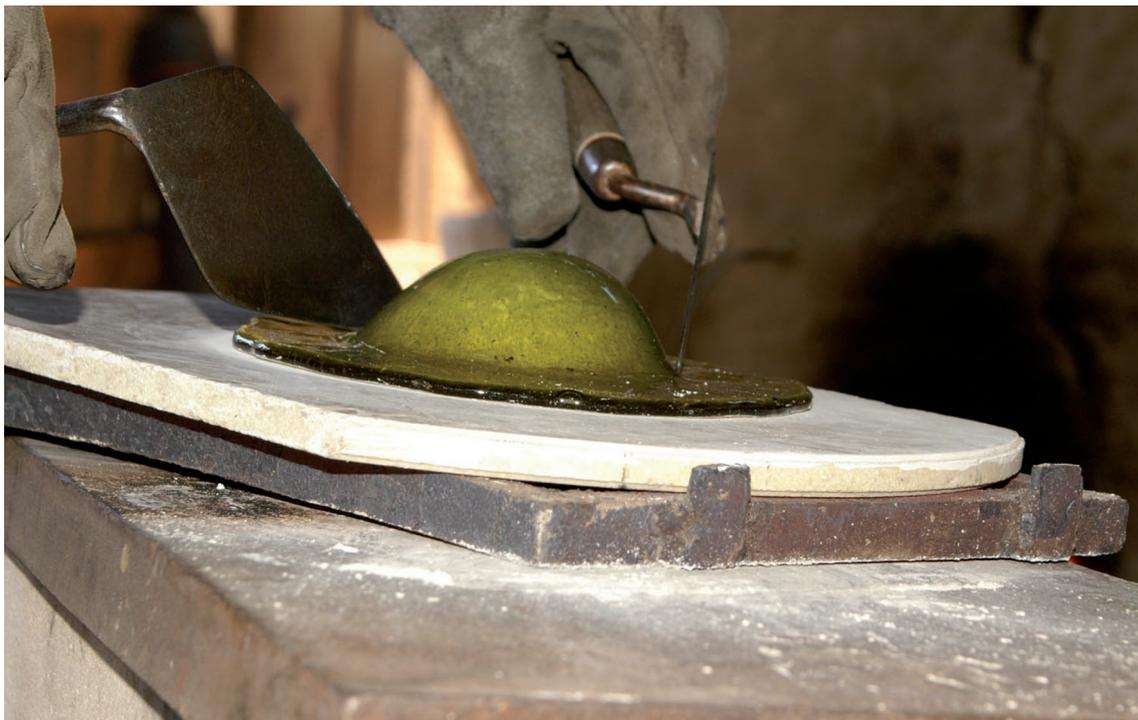
Fig. 8: Last corrections of the domed window glass.
