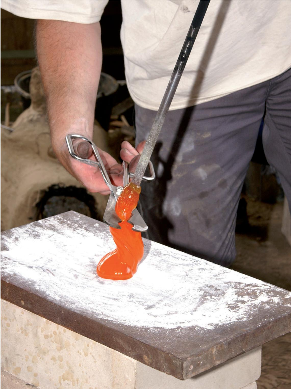
Fig. 2: Placing the hot gather of glass.
