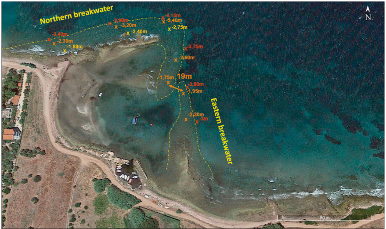
Fig. 9 Measures of the breakwaters and of the entrance of the harbour of Anthedon. – (Photo A. Ginalis, 2018).
