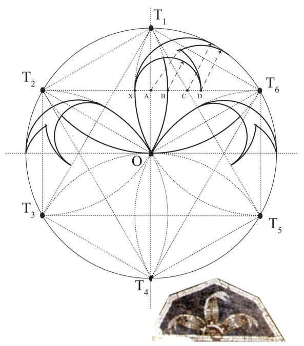
Fig. 3: Geometric Drawing of the Triple Leaf Pattern.
