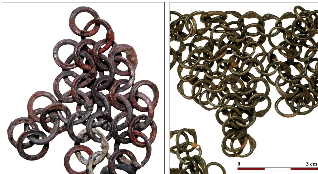
Fig. 5: Left: Roman mail always consists of solid and clockwise riveted rings: an example comes from Künzing 2 in Germany, dated to AD 200–244. Right: mail fragment from Thorsberg 14 in northern Germany (AD 200–250) made entirely of anti-clockwise riveted rings.
