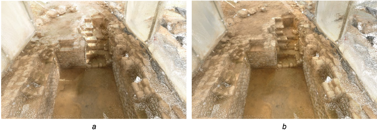
Fig. 8. Comparison of the results based on a point cloud rendering: colorization a) without and b) with the exposure problem detection (© Arnaud Schenkel).
