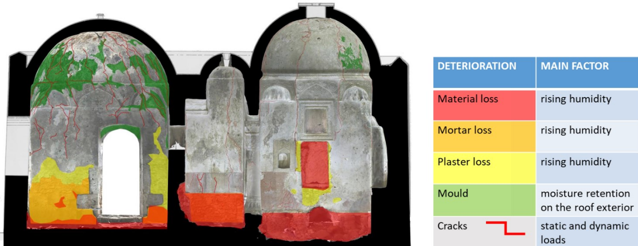
Fig. 4. Section -Main Deteriorations.
