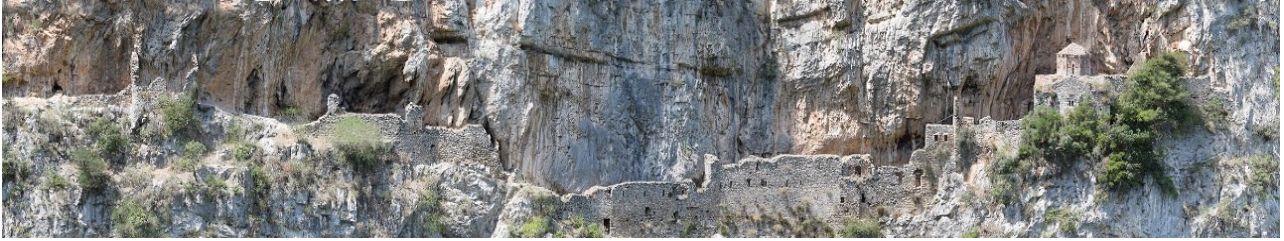
Fig. 1. Orthophotomosaic / Facade of Old Philosopher's Monastery (© IMANTOSIS [2014]). Details of original Orthophotomosaic: accuracy 1cm / pixel size 3 mm / more than 300 physical targets all measured by robotic total station & 3D Scanner. Processed & Produced in Agisoft Photoscan Software.
