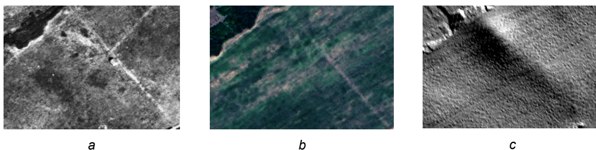
Fig. 1. Via del Sabazeo, Ostia Antica: a) historical aerial photo (SARA, 1930 c.); b) GeoEye01, July 6, 2015, RGB (© DigitalGlobe); c) Hillshade LiDAR A45-H10-Ve2.0.
