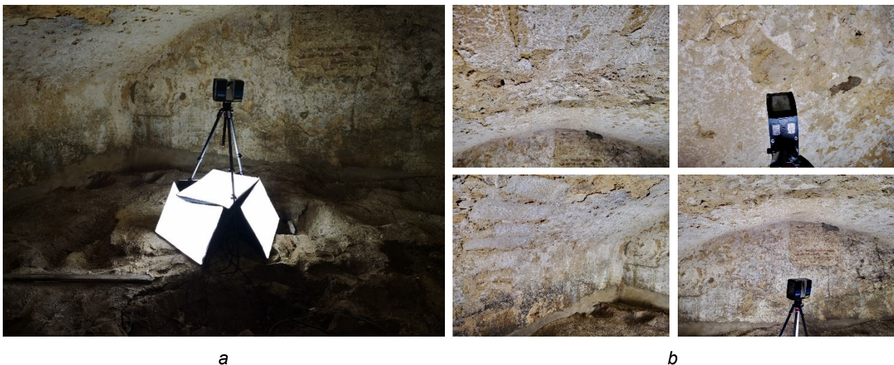
Fig. 2 a) Lighting equipment prototype, placed in a cellar where no natural light illuminates the surfaces, and b) some pictures of the surrounding elements lit with it (© PANORAMA).
