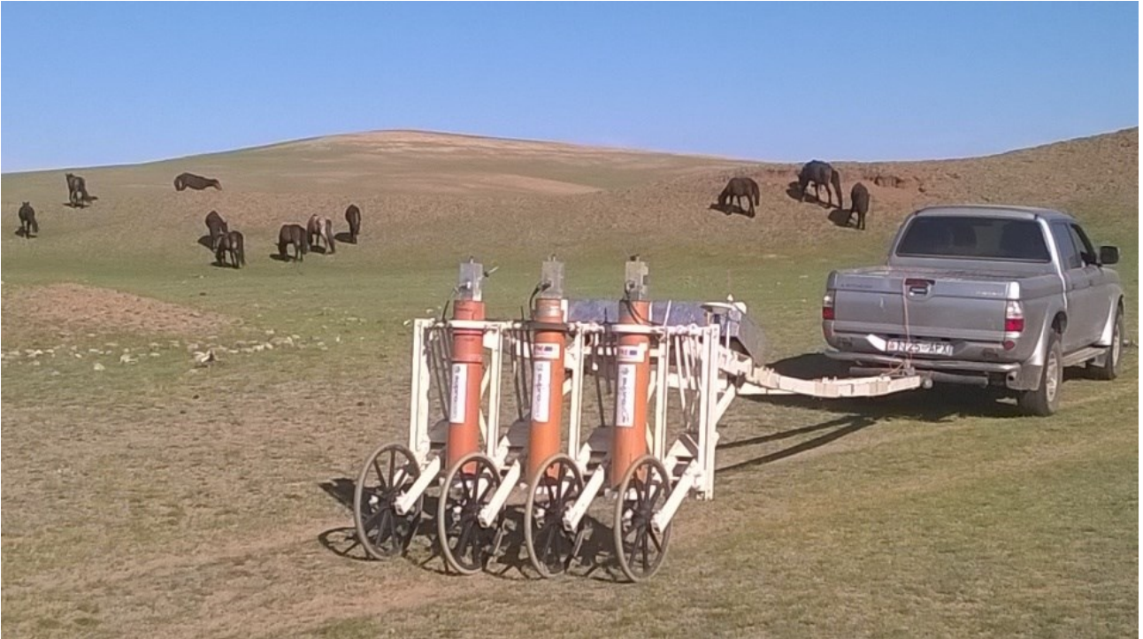
Fig. 1. The SQUID measuring system in operation nearby the main walled enclosure of Khar Khul Khaany Balgas, Mongolia. The three orange cryostates contain 18 magnetic field sensors within a scanning width of 1.5 metre (© Sven Linzen, Leibniz IPHT).
