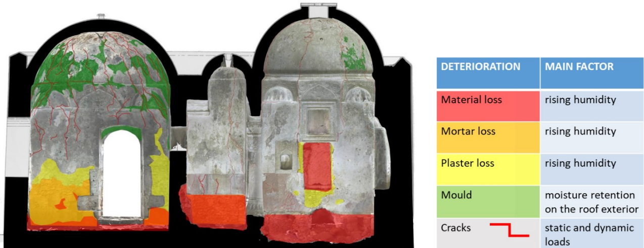
Fig. 4. Section -Main Deteriorations.
