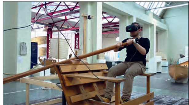
Fig. 15 Interaction between real and virtual world: the connection of the replica of an oar section with the virtual ship allows a true-to-life impression of the oar action. Weights on the oar simulate the felt resistance of the water. Remigatio Project in the context of a Bachelor thesis at the Hochschule Mainz, 2019. – (Photo A. Franz).
