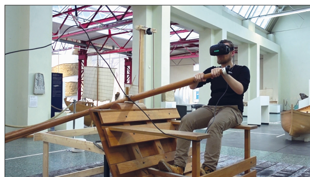
Fig. 15 Interaction between real and virtual world: the connection of the replica of an oar section with the virtual ship allows a true-to-life impression of the oar action. Weights on the oar simulate the felt resistance of the water. Remigatio Project in the context of a Bachelor thesis at the Hochschule Mainz, 2019. – (Photo A. Franz).
