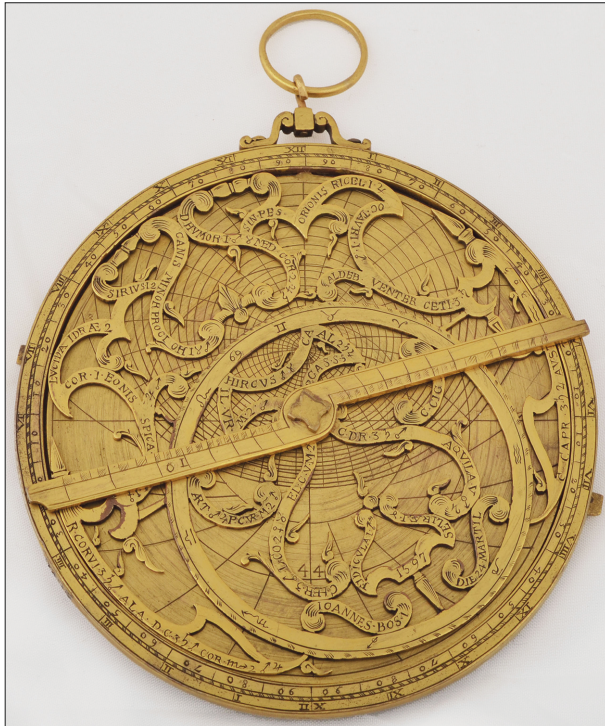
Fig. 1 Astrolabe, signed »Ioannes Bos I / 1597 / Die 24 Martii«, acquired by R. S. Whipple from the Parisian dealer Gertrude Hamilton (trading as »Mercator«) in 1928. It is now known that a near-identical astrolabe in the Adler Planetarium (carrying the same inscription) is authentic, while five other similar instruments, including this one, are fake. – (Image © Whipple Museum of the History of Science, University of Cambridge [Wh.0305]).
