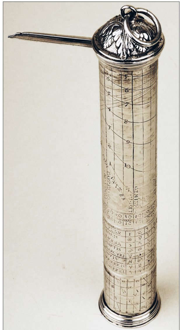
Fig. 4 Silver pillar dial with sand caster, signed »CHRITOPHURUS [sic] SCHISSLER FECIT '79«, but actually almost certainly a modern fake, c. 1935. – (Image © Whipple Museum of the History of Science, University of Cambridge [Wh.0776]).
