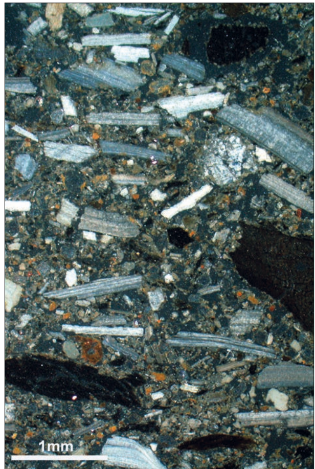
Fig. 3.46 MM2 (as fig. 3.45), under OIL; white shell is clearly burnt. – Scale bar 1 mm.
