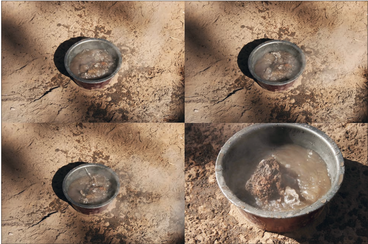
Fig. 2.52 Experimental speleothem; gentle placing (not dropping) into water was followed by almost immediate boiling, persisting for over 2 minutes. – Bowl diameter 22 cm.
