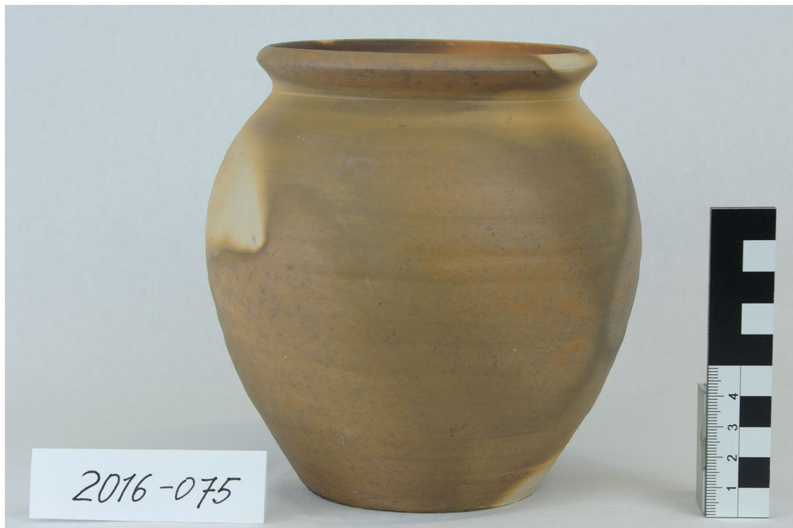
Fig. 8: Experimental pot after going through ten rounds of thermal shock testing. Inv.-Nr. 2016-075, Clay: MV4/ White 50% – Red 50%.
