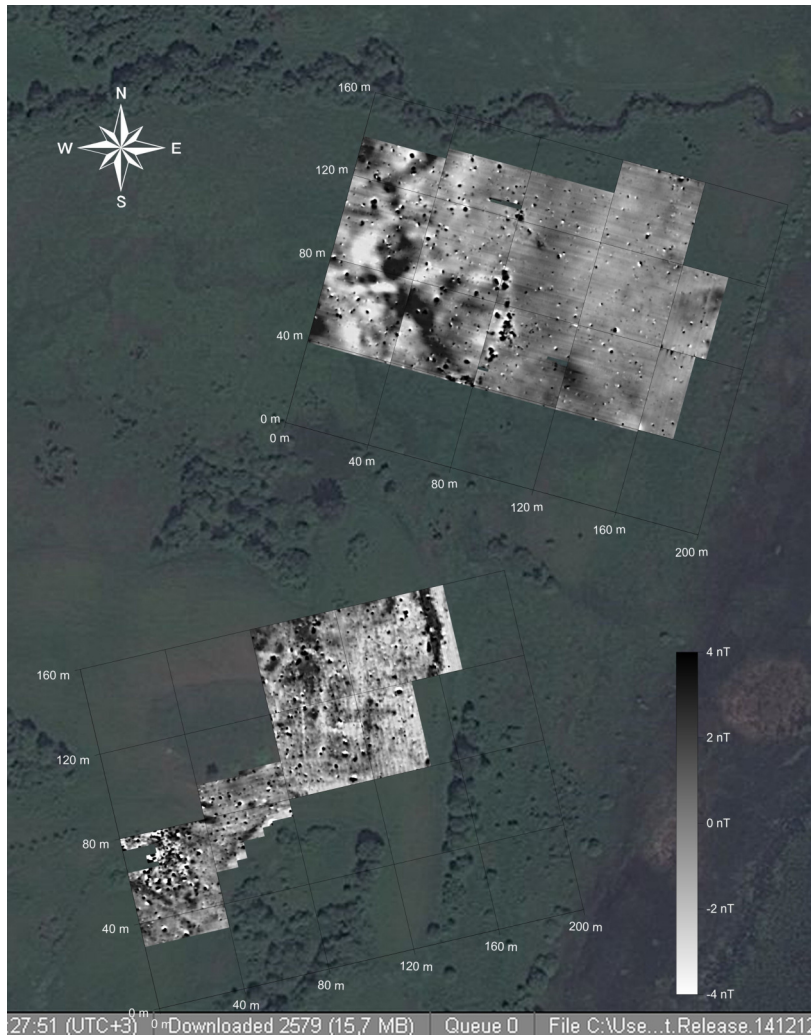
Figure 12: Dubokray. Satellite image overlaid by the magnetogram images from 2013 and 2016 of the site as a grey shade plot. Cesium-Smartmag SM4G-special-magnetometer, duo-sensor configuration, sensitivity \pm 10 pT, sampling interval 12,5 x 50 cm interpolated to 25 x 25 cm in 40 m grid. Total field values were reduced to the mean value of a 40 m square and partly fused by a high-pass filter magnetogram, dynamics \pm 4 Nanotesla from black to white.
