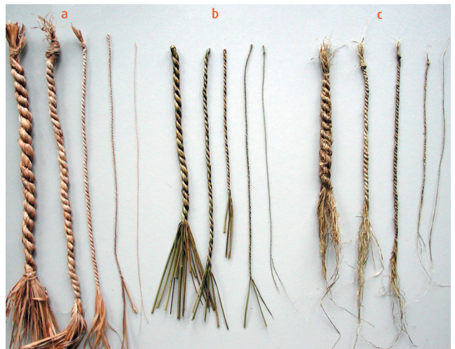
7 Zwirne verschiedener Dicke aus Lindenbast (a), Binsen (b) und Brennesselfasern (c). • Twined cords of various thicknesses made of lime bast (a), rushes (b) and nettle fibres (c).
