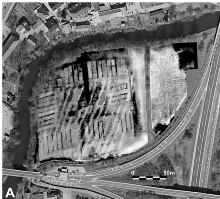
Fig. 4: Geoelectric mapping image of market square and horrea at Nauportus.
