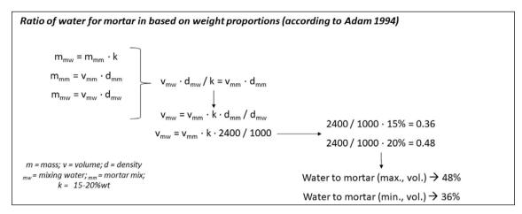
Fig. 4: Calculations for the ratio (percentage) in volume between fresh mortar and the water necessary to mix it, given an ideal mix of putty to sand (1 : 3 vol), where the putty was slaked in a 1 : 3 (wt) mix.
