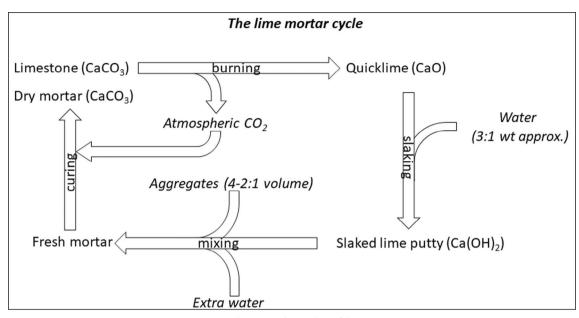
Fig. 2: The chemical cycle of lime mortar.
