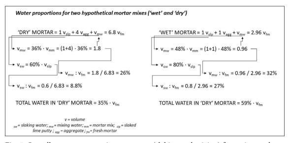
Fig. 5: Overall water consumption necessary (slaking and mixing) for a given volume of fresh mortar.
