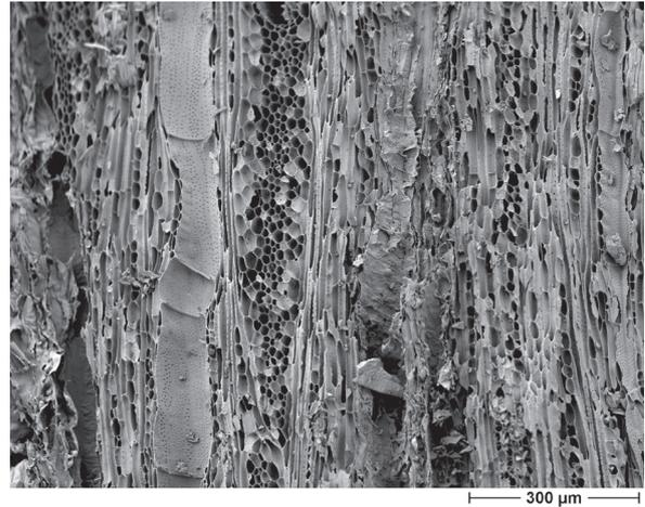
Fig. 12 *Leptadenia pyrotechnica* wood charcoal, tangential section, SEM.
