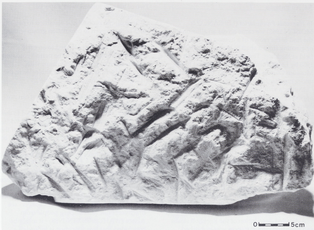
Fig. 32 Pick marks on chalk slab originating from the ceiling of a gallery in mine Nr. 8.
