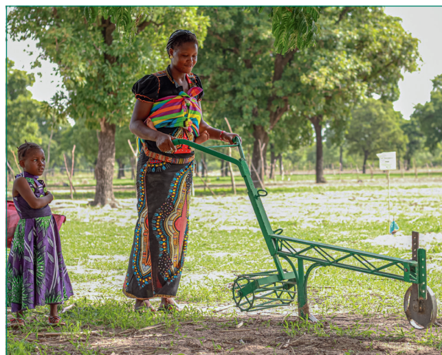
Fig. 2 The in-line strip tiller loosened and firmed the soil in a narrow planting zone, retaining protective crop residues between the rows (Picture: Maria Jones).
