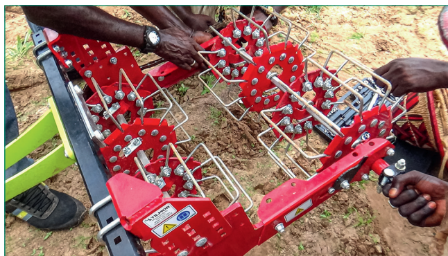
Fig. 9 Modern weeding tools can be adapted for animal traction. This basket weeder, coupled with a finger weeder and spyders, works well within and between the rows (Picture: T. Harrigan).
