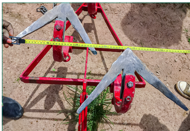
Fig. 7 Low-crown, low-pitch cultivator sweeps under-cut weeds and loosens the soil, reducing cultivator draft and improving weed control (Picture: T. Harrigan).
