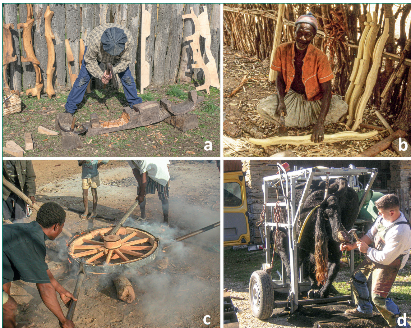
Fig. 15 Examples of artisanal support services needed for draft cattle. a). Demonstration of French yoke making. b). Yoke making in Guinea. c). Cartwheel making in Madagascar. d). Shoeing a draft ox in France (all: P. Starkey).
