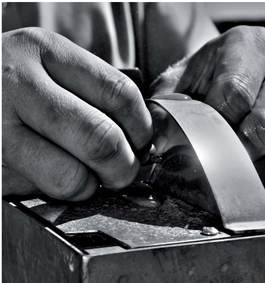
Figure 5. Cutting of finds at Tell el-Farkha to reveal fresh metal surfaces (photo by M. JÓRDECZKA).
