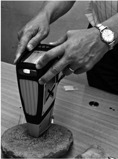
Figure 4. Analysis of a stone tool using pXRF at Tell el-Farkha (photo by M. JÓRDECZKA).
