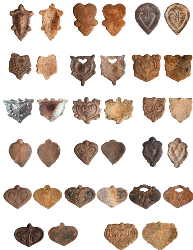
Fig. 10 Lead models of sand-casting. – (Photos S. Doncheva).
