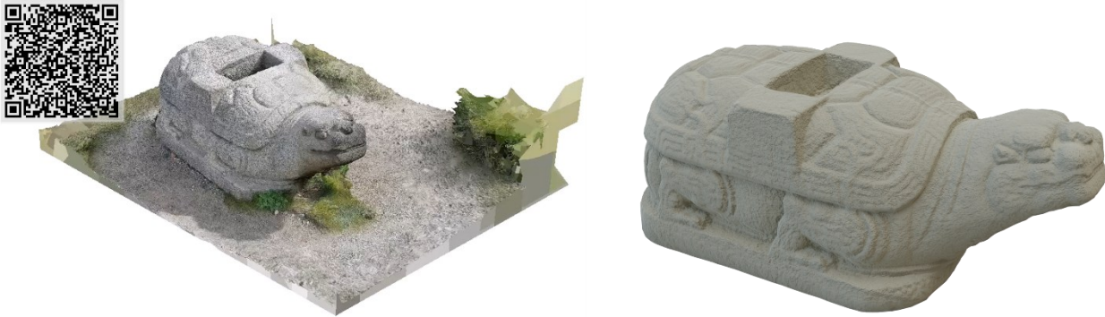
Fig. 4. On the right is the high-poly model from RealityCapture with around 12 Million vertices and 1.9 GB in file size and on the left the AR-compatible low-poly model with only ten thousand vertices and 1.7 MB in file size (here without the color texture). Both, the vertice count and the file size could be significantly reduced. (© High-poly model: Marco Block-Berlitz/DAI; Low-poly model: Lukas Suthe/DAI).
