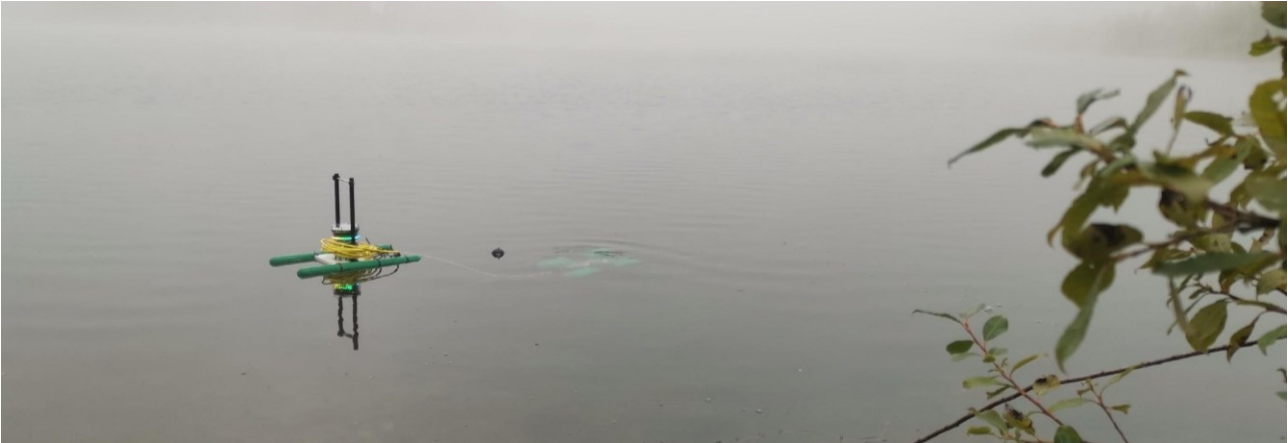
Fig. 1. Current system with the Buoy above water connected via a yellow cable with the submarine underwater. (© M. Bommhardt-Richter).
