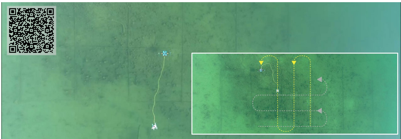
Fig. 2. The recording strategy under water is comparable to that above water. Here, however, the degrees of freedom of the submarine and the cable it carries play an important role in the recording rate. (© M. Block-Berlitz).
