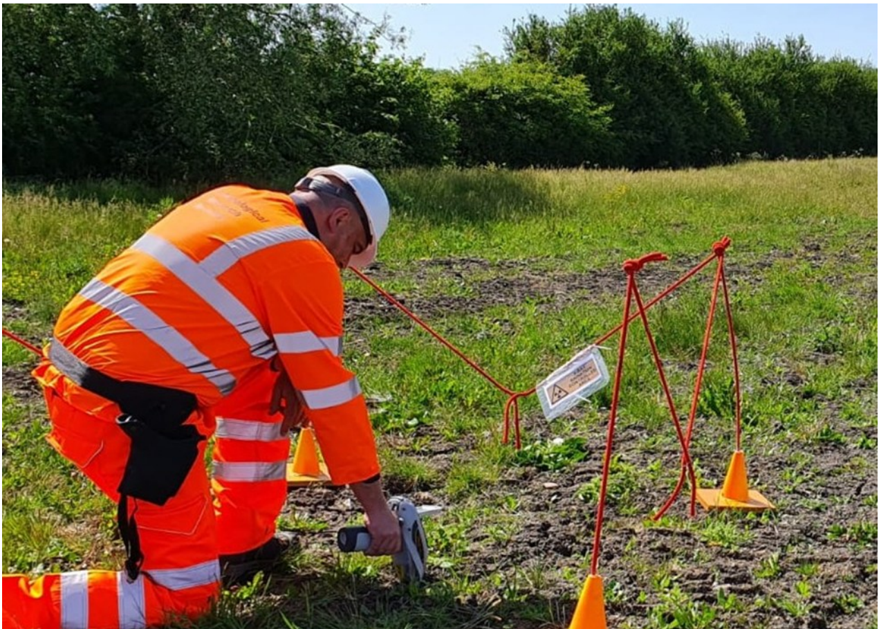
Fig. 1. A geochemical analysis being undertaken in the field using a portable XRF instrument (© Fusion JV).
