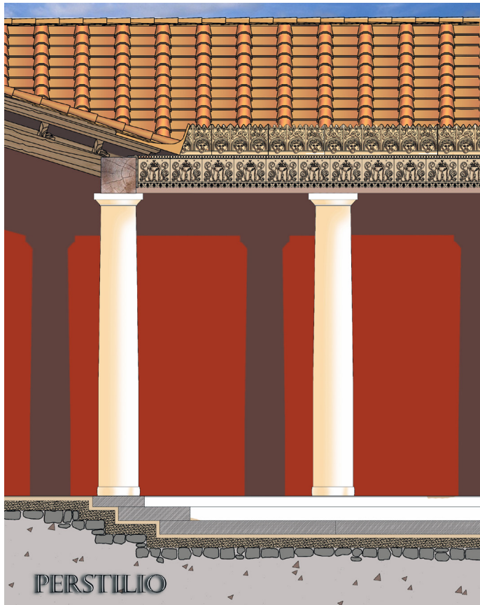
Fig. 4 Reconstruction of the peristyle of the Cottanello villa showing architectural terracottas on the entablature and eave (A. D'Eredità).
