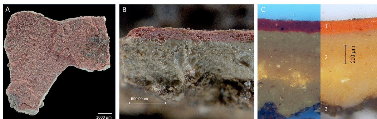
Fig. 6 Clay plaster fragment Type 2, Burial CG5: A top view of painted side, B profile with three layers, C polished cross-section in UV and polarised light. (Photos: N. Reifarth, U. Drewello)
