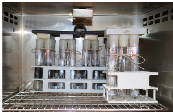
Fig. 12 Airtight glass tubes for the Oddy Test. Eleven different materials were tested to prove whether they are suitable for mounting. (Photo: A. Costes)
