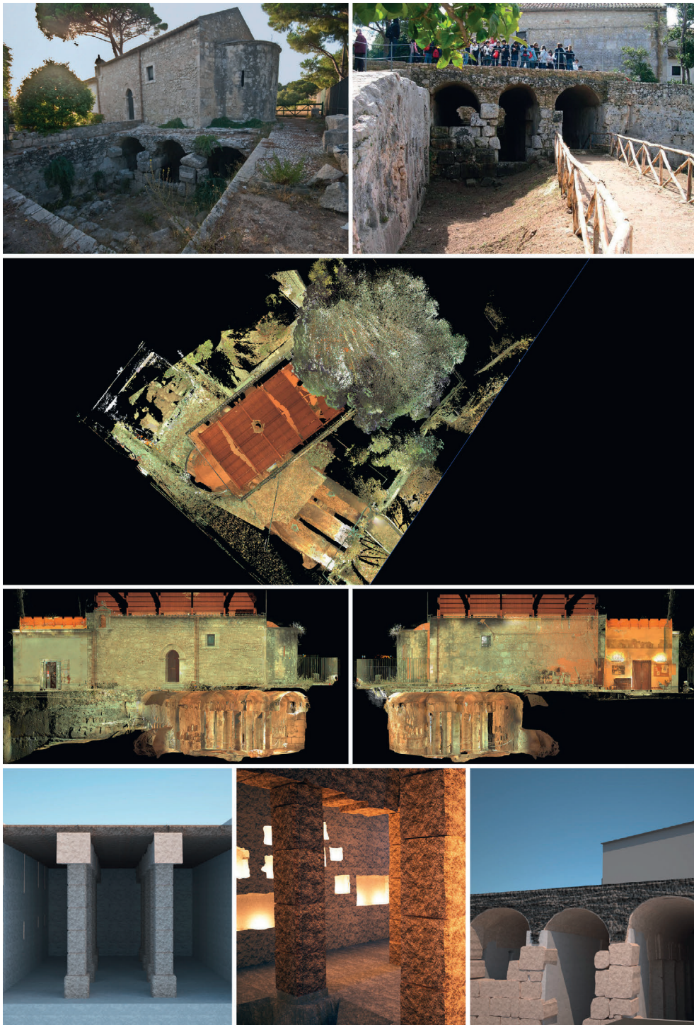
Fig. 5 Syracuse. The Archaeological Park of Neapolis. Roman Pool. Survey TLS, virtual reconstruction and life cycle restitution. Images processed by Laboratory of Representation of SDS of Syracuse, University of Catania.
