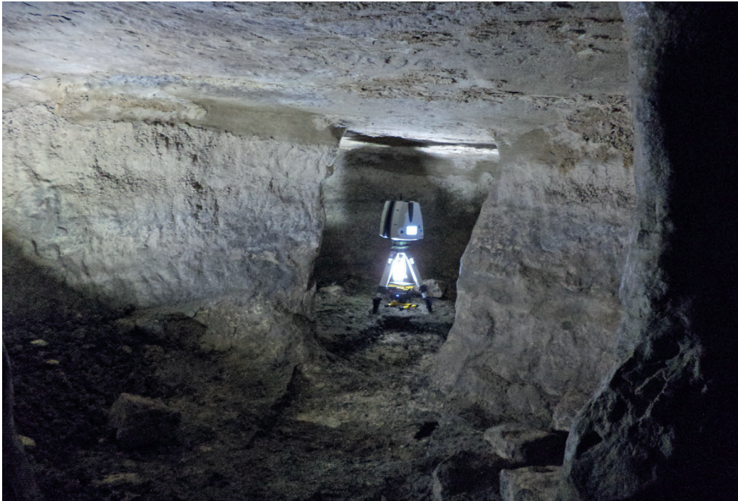
Fig. 7 The laser scanner activity into the hypogeum (photo by the author).
