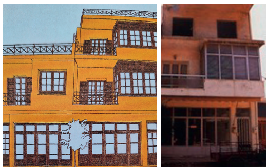
Fig. 31 Changing the aspect of modern constructions in order to comply with the notion of traditional architecture. (Source: Acts Archanes 1992: 172)
