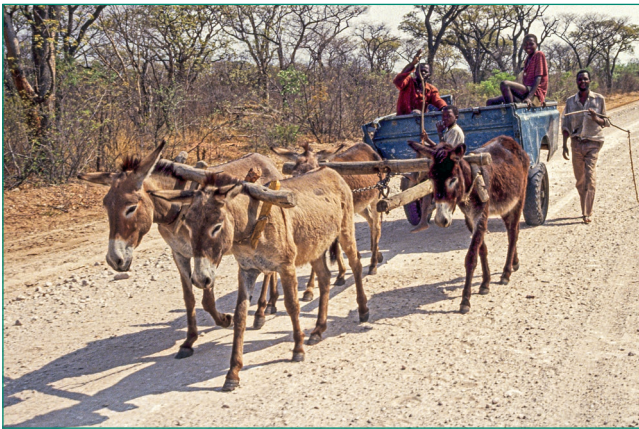
Figure 20 – Four donkeys, harnessed in pairs with yokes, pulling a donkey cart in Namibia
