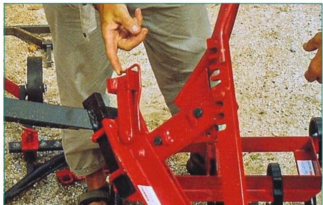
Figure 11 – Process of changing a tool: Pull the lever up
