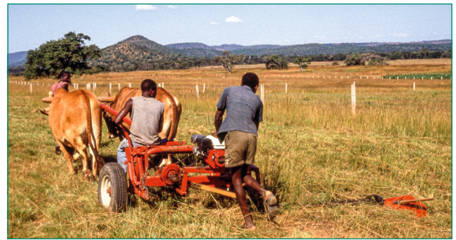
Figure 13 – Wheeled toolcarrier fitted with a motorised grass cutter on a research station in Zambia
