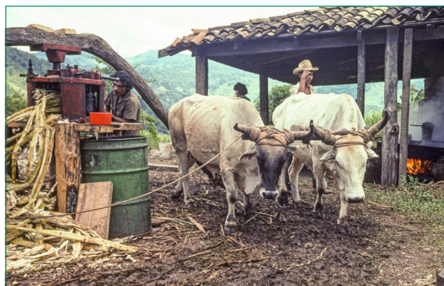
Figure 20 – Oxen turning ‘trapiche’ mill to crush sugar cane in Honduras
