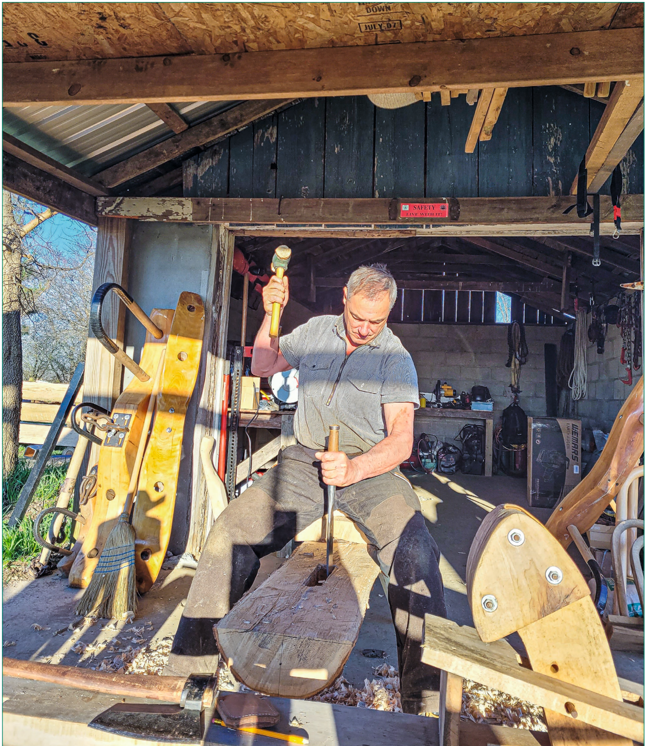
Figure 4 – Part of our woodland management strategy is to utilize all the products we harvest; here, low grade red oak is being fashioned using simple hand tools into useful tools such as these shaving horses which will then be utilized to teach green woodworking
