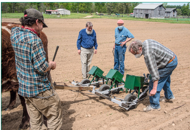
Figure 16 – Field-testing a three-row, ox-drawn planter at Tillers International
