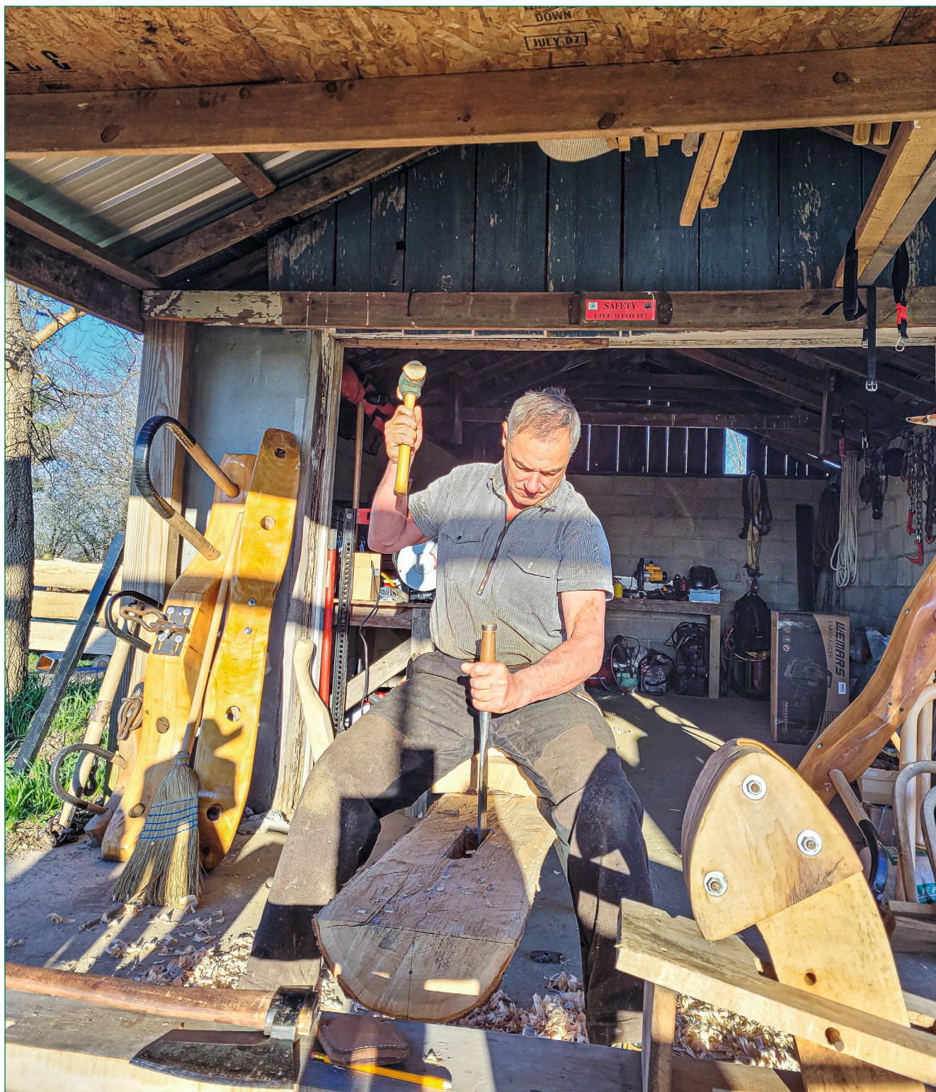
Figure 4 – Part of our woodland management strategy is to utilize all the products we harvest; here, low grade red oak is being fashioned using simple hand tools such as these shaving horses which will then be utilized to teach green woodworking
