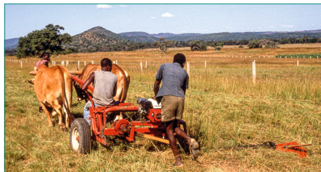
Figure 13 – Wheeled toolcarrier fitted with a motorised grass cutter on a research station in Zambia
