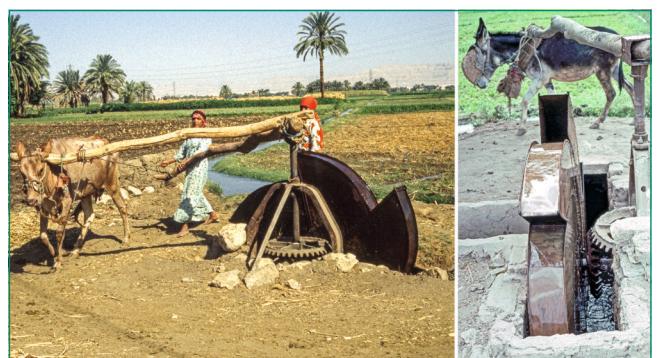
Figure 21 – Raising irrigation water using a sakia in Egypt with a cow (left) and a donkey (right)
