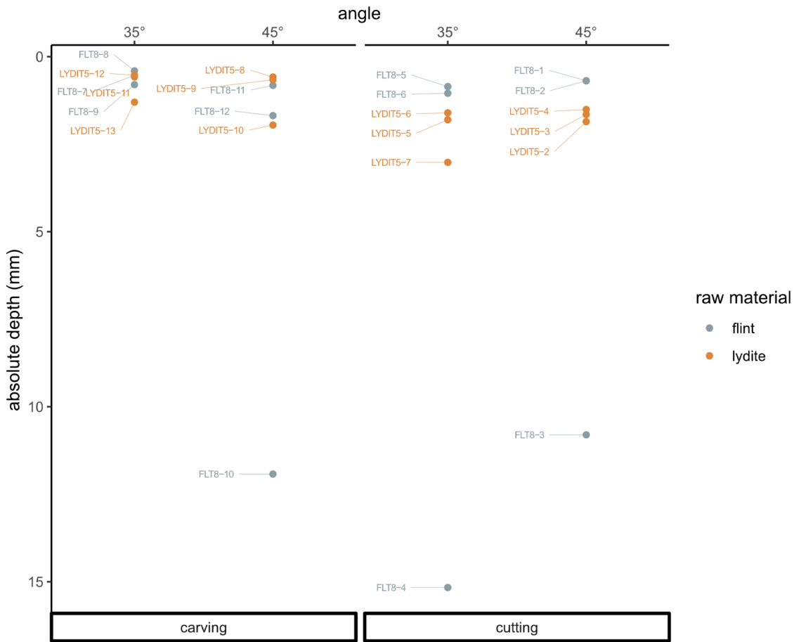
Fig. 147 Absolute cutting depth of all samples used during the tool function experiment. The samples are organised according to the performed task and the edge angle of the standard sample.
