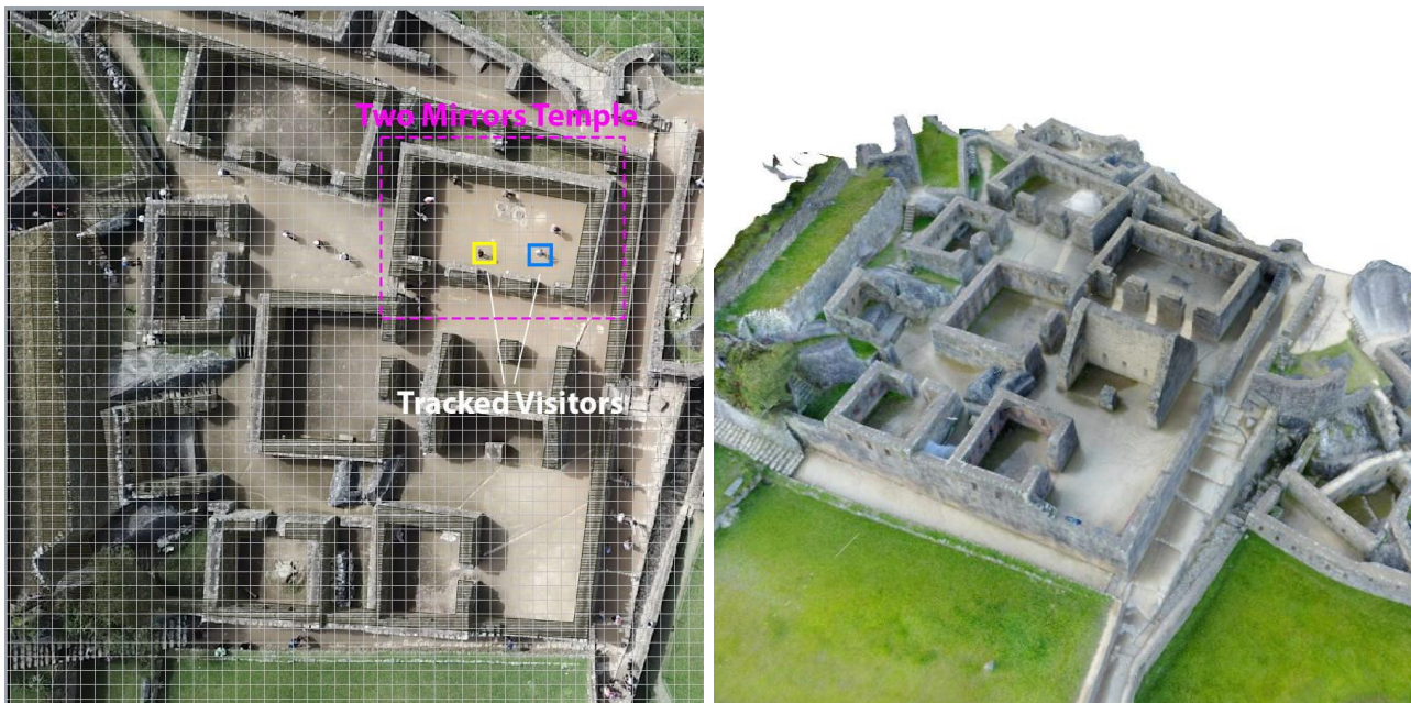
Fig. 2. Right: Two Mirror Temple area in Machu Picchu is captured into a photogrammetric model (Nagakura, 2018). Left: The pedestrians marked with yellow and blue boxes near the entries of the 'two mirrors' site are being tracked in the video recorded from a drone. © Authors.
