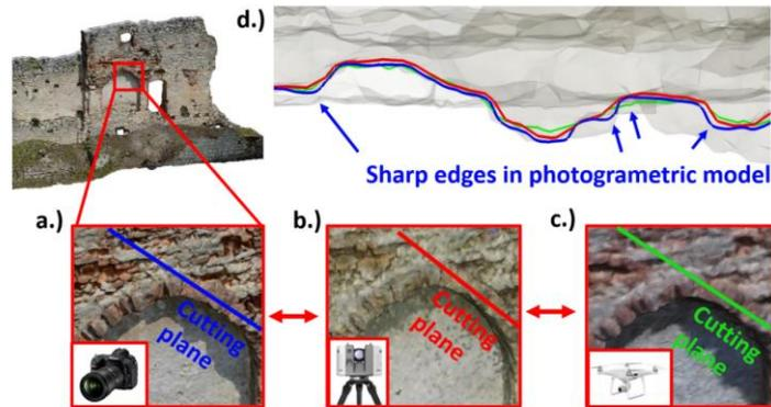
Fig. 2. Comparison between the different observation methods a) SLR model b) TLS model c) UAV model d) by using geometric cutting lines through the obtained 3D models
