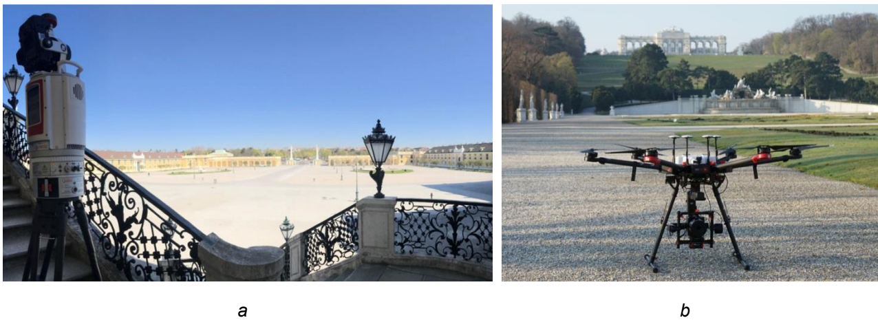
Fig. 1. a) TLS RIEGL VZ-400i placed on the main staircase of the northern courtyard of Schönbrunn palace. The TLS and the on-top mounted camera have been used to capture a high resolution, colour coded point-cloud of the facades; b) DJI Matrice 600 pro with Phase One iXM-100 medium format camera as used for capturing high-resolution stereo-photos of the roof area. © Authors.
