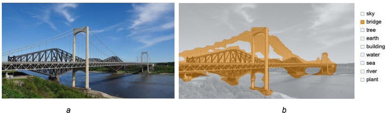
Fig. 3. Machine vision identification of bridge and other features a) original image; b) identified features. (Image source: a) https://commons.wikimedia.org/wiki/File:LaPorte_de_Quebec_(5802230245).jpg , b) Created by W. J. Turkel using Ademxapp Model A1
