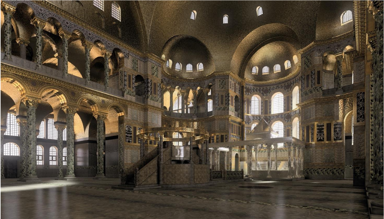
Fig. 1. A visualisation of Hagia Sophia's interior in the sixth century accounting for contrast and brightness based on day-light simulation. The simulation environment includes a reconstruction of the historic geometry and the optical properties of the surfaces. The environment is associated with a multitude of research data. © Authors.
