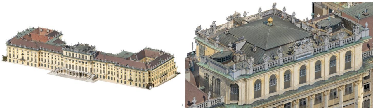
Fig. 4. Textured 3D-model of Schönbrunn Palace combining the TLS point-cloud at the façade area and a textured 3D-triangulation model of the roof structure. © Authors.
