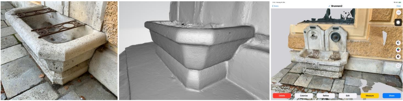
Fig. 6. Result of the complementary data acquisition using the iPhone-LiDAR sensor. f.l.t.r.: Original picture from iPhone; triangulation mesh from iPhone LiDAR sensor; textured 3D-mesh. © Authors.
