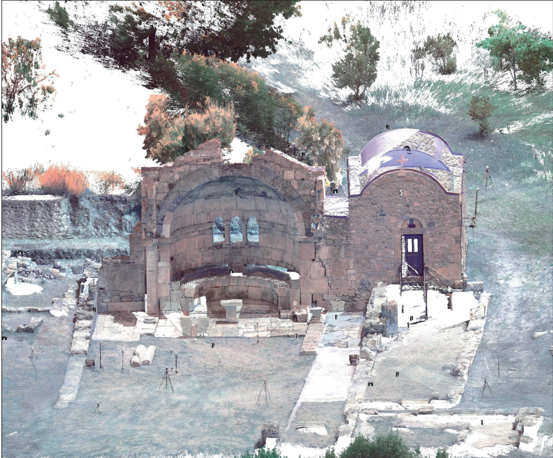
Fig. 6: Point cloud (incomplete) of the basilica of Christ of Jerusalem and the Chapel of Ypakou.
